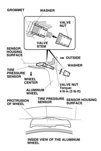
7. While holding the tire pressure sensor to keep it from rotating, torque the valve nut to 4 N·m (3 lb-ft). You may hear a snap or pop as you torque the nut; this is normal.
