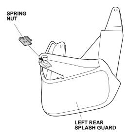
9. Loosely install the left rear splash guard to the left rear inner fender with two 5 x 16 mm self-tapping screws and one self-tapping screw.
