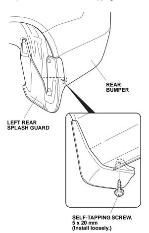
11. While holding the left rear splash guard against the rear bumper, tighten the four self-tapping screws in the order shown. Make sure there is no gap or looseness between the left rear splash guard and the vehicle. If there is, loosen the four self-tapping screws, adjust the splash guard to remove the gap or looseness, and retighten the screws.
