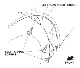
7. Secure the left bracket on the left rear inner fender with two self-tapping screws.
