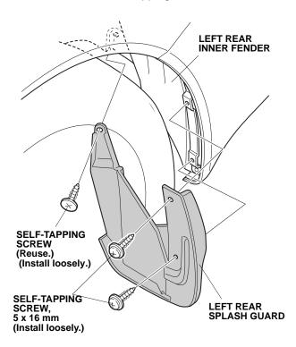
10. Loosely secure the left rear splash guard to the rear bumper with a 5 x 20 mm self-tapping screw.
