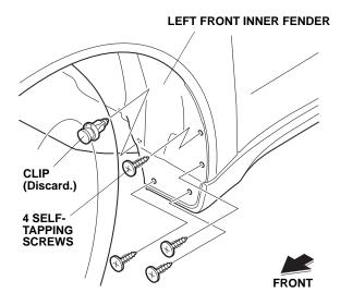
2. Remove the four self-tapping screws and one clip from the left front inner fender.
