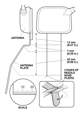
26. Starting at the antenna end of the cable, wrap three urethane tapes around the antenna cable at the measurements shown.
