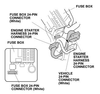
46. Attach the clip on the engine starter harness 24-pin connector to the clip holder on the bottom of the fuse box as shown.
