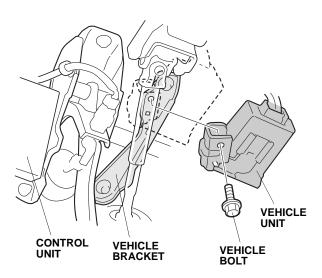
56. Attach the engine starter harness clip to the vehicle bracket.
