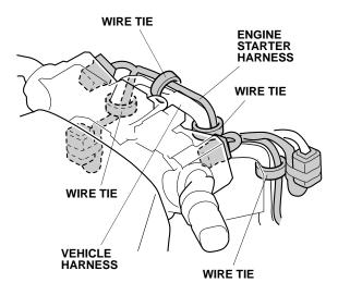
64. Secure the engine starter harness to the vehicle harness with one wire tie.
