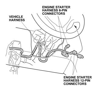
60. Route two 12-pin connectors and two 8-pin connectors on the engine starter harness along the vehicle harness as shown.
