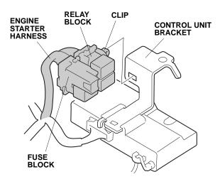
44. Remove the vehicle nut from the vehicle bracket, and secure the control unit bracket to the vehicle bracket with one flange nut and one vehicle nut.
