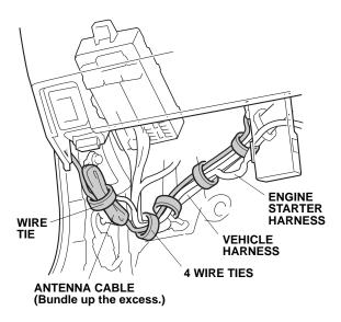
54. Bundle up the excess antenna cable as shown, and secure it to the vehicle harness with one wire tie.
