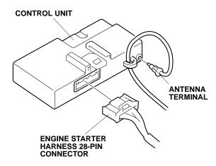
41. Plug the engine starter harness 28-pin connector into the control unit.
