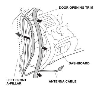
36. Route the antenna cable along the vehicle harness as shown.
