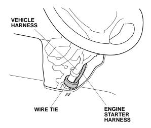
65. Secure the engine starter harness to the vehicle harness with two wire ties as shown.
