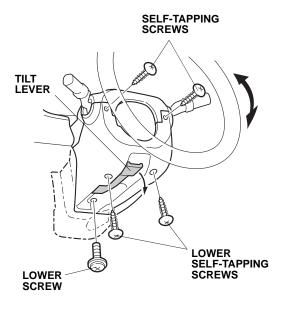
8. Turn the steering wheel as necessary to access each self-tapping screw, and remove the two self-tapping screws.
