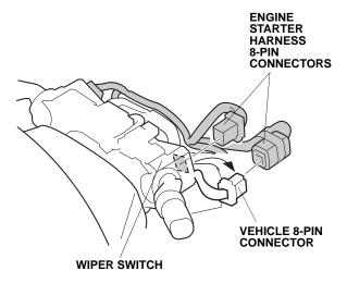
63. Secure the engine starter harness to the vehicle harness with four wire ties. Do not secure it to the SRS harness.
