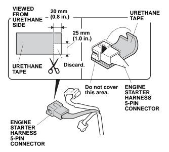
49. Unplug the vehicle 5-pin connector from the fuse box, and plug it into the engine starter harness 5-pin connector. Plug the remaining engine starter harness 5-pin connector into the fuse box 5-pin connector.
