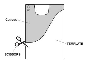
24. Using masking tape, attach the template to the windshield. Align with the black ceramic as shown.
