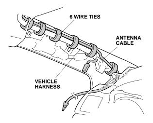
35. Pull away the door opening trim from the left front A-pillar. Route the antenna cable down next to the dashboard, and tuck the antenna cable between the left front A-pillar and the dashboard. Reinstall the door opening trim.
