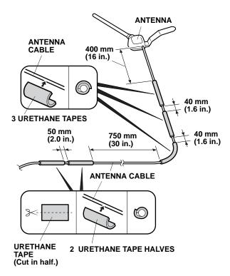
27. Using scissors, cut one urethane tape in half. Wrap the two halves of the urethane tape around the antenna cable at the measurements shown.
