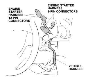
61. Unplug the vehicle 12-pin connector from the turn signal switch, and plug it into the engine starter harness 12-pin connector. Plug the remaining engine starter harness 12-pin connector into the turn signal switch.
