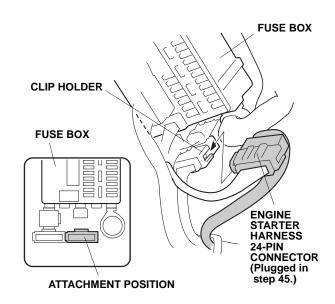
47. Unplug the vehicle 20-pin connector (Green) from the fuse box, and plug it into the engine starter harness 20-pin connector. Plug the remaining engine starter harness 20-pin connector into the fuse box 20-pin connector.
