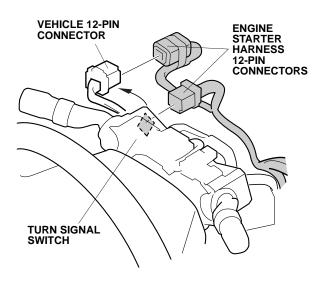
62. Unplug the vehicle 8-pin connector from the wiper switch, and plug it into the engine starter harness 8-pin connector. Plug the remaining engine starter harness 8-pin connector into the wiper switch.
