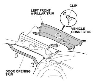
18. Remove and discard the clip from the left front A-pillar trim, and install a new A-pillar clip (supplied).
