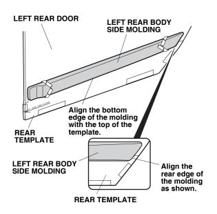
12. Press on the left rear body side molding firmly with the palm of your hand while removing about 2 to 4 inches of the adhesive backings at a time.
