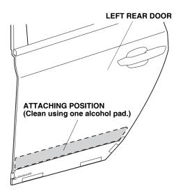
11. Align the edges of the left rear body side molding with the edges of the rear template as shown, then install the left rear body side molding on the left rear door.
