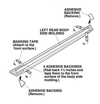
10. Clean the door surface where the left rear body side molding will attach using one alcohol pad. Allow the alcohol to dry.
