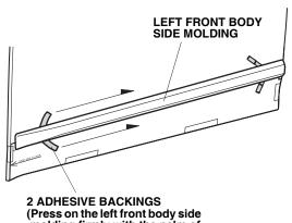
(Press on the left front body side molding firmly with the palm of your hand while removing the adhesive backings)
