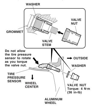
3. Torque the valve nut to 4 N·m (36 in-lb) while holding the tire pressure sensor toward the wheel. You may hear a snap or pop as you tighten the nut-this is normal.
