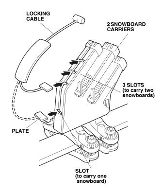
14. After loading the snowboards on the carrier, adjust them with the help of the board supports so that the top edges are level and the boards are as far down in the carrier as possible. To secure the snowboards, use the key to open the covers, then insert the locking cable barrels into the holes in the carrier covers.
