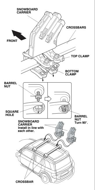
8. Turn the knobs on the top clamps to tighten the snowboard carrier.
