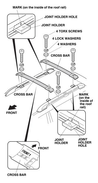
5. Position the cross bars on the joint holders, and install four TORX screws with four washers and four lock washers. Tighten the TORX screws securely.
