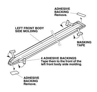
4. Position the left front body side molding on the left front door, and align it with the two marks made in step 2.
