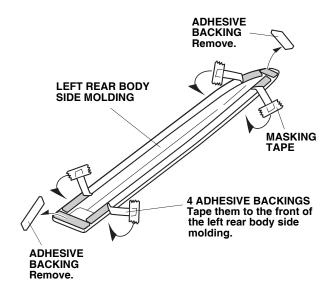
10. Position the left rear body side molding on the left rear door, and align it with the two marks made in step 8.
