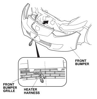
25. Secure the heater harness to the front bumper grille with four black wire ties.
