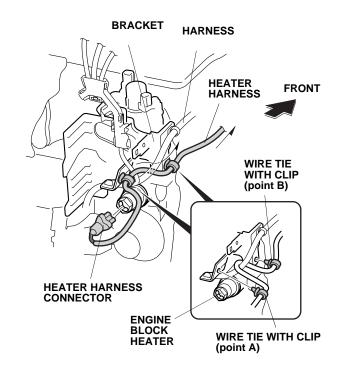
18. Route the heater harness as shown, and secure the wire tie with clip (point C) to the vehicle frame.
