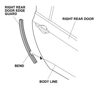
Using a felt-tip pen, mark the inside edge of the right rear door at the upper and lower ends of the right rear door edge guard.
