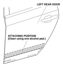
Align the edges of the left rear body side molding with the edges of the rear template as shown, then install the left rear body side molding on the left rear door.
