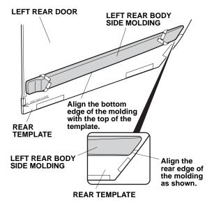
12. Press on the left rear body side molding firmly with the palm of your hand while removing about 2 to 4 inches of the adhesive backings at a time.
