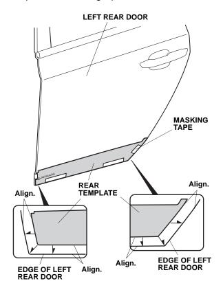
Peel back approximately 1-1/2 inches of the adhesive backing from each adhesive tape, and tape the ends to the front surface of the left rear body side molding. Remove the small end pieces of adhesive backing.
