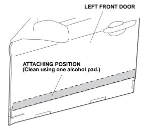
Align the edges of the left front body side molding with the edges of the front template as shown, then install the left front body side molding on the left front door.
