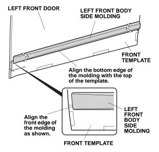
5. Press on the left front body side molding firmly with the palm of your hand while removing about 2 to 4 inches of the adhesive backings at a time.
