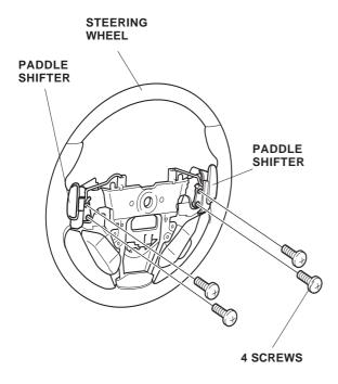
11. Remove the steering trim and unplug the two switch connectors.
