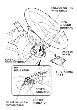
Unplug the airbag connectors. While holding the pin insulator, pull out on the cover insulator. Do not pull on the socket insulator and harness wires.  Remove and discard the two TORX bolts that secure the airbag, and remove the airbag.
