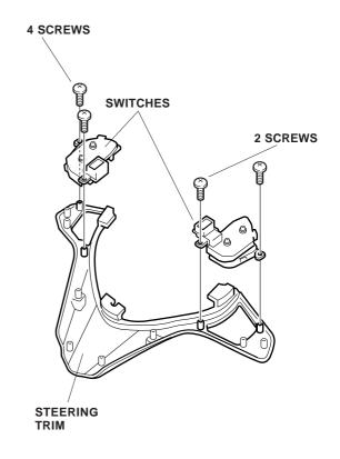
13. Install the two switches to the new steering trim with the four screws you removed.
