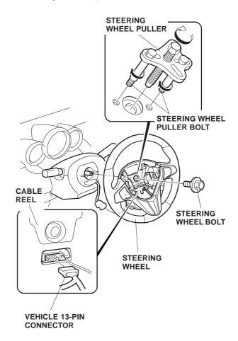
8. Remove the steering wheel bolt. Disconnect the vehicle 13-pin connector from the cable reel. Using a steering wheel puller, remove the steering wheel. Do not thread the steering wheel puller bolts in more than 10 mm. Be careful not to turn the steering wheel during removal.
