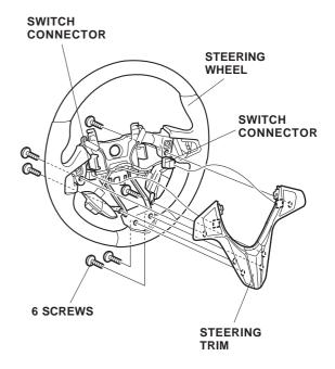
12. Remove the switches from the steering trim (two screws for each switch).
