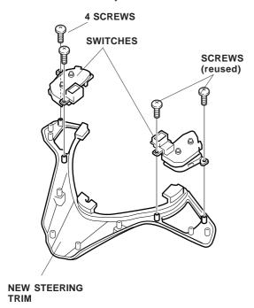
Install the new steering trim to the steering wheel with the six screws and connect the two switch connectors.
