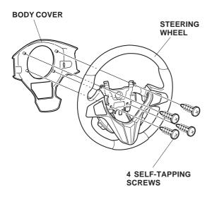
10. Remove the four self-tapping screws that fasten the paddle shifters to the steering wheel.
