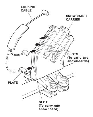
15. After loading the snowboards on the carrier, adjust them with the help of the board supports so that the top edges are level and the boards are as far down in the carrier as possible. To secure the snowboards, use the key to open the covers, and insert the locking cable stops into the holes in the carrier covers.
