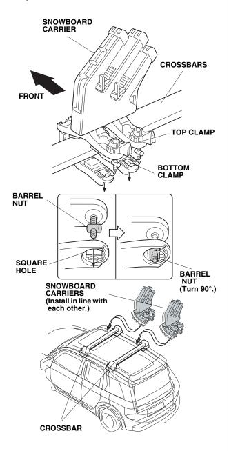
8. Turn the four knobs on the four top clamps to tighten the snowboard carrier.
