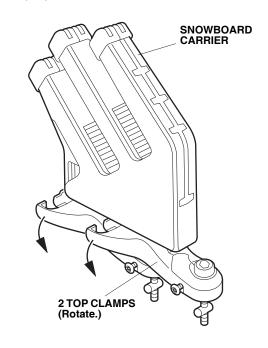
2. Install two board supports to the snowboard carrier.
