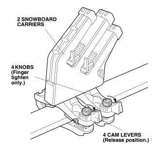
9. Return the four cam levers to the original locations (turn clockwise).
