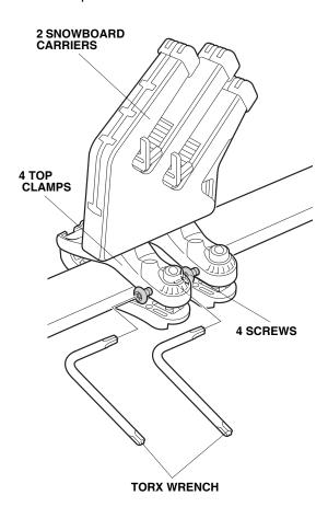
11. Try to move the two snowboard carriers and make sure they are securely installed.
