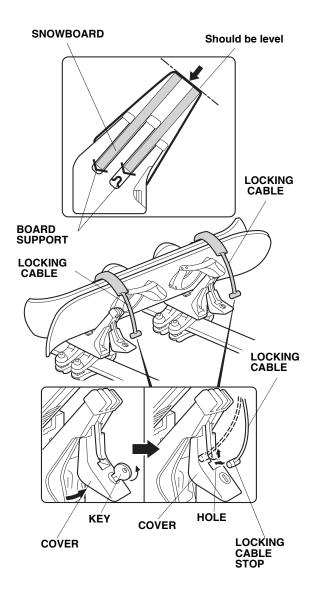
14. Check that the locking cables are installed securely, then close the covers.
