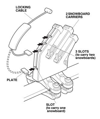
13. After loading the snowboard(s) on the carrier, adjust it (them) with the help of the board supports so that the top edges are level and the boards are as far down in the carrier as possible. To secure the snowboard(s), use the key to open the covers, then insert the locking cable stops into the holes of the carrier covers.
