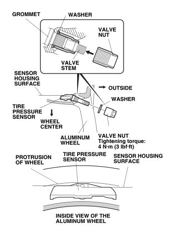
Install the tire pressure sensor:
