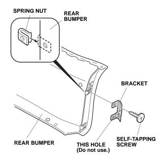
8. Attach the bracket to the rear bumper using one selftapping screw. 9. Peel back approximately 1-1/2 inches of adhesive backing from each adhesive tape, and tape the ends to the front surface of the left rear under spoiler.
