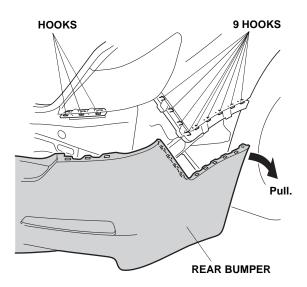
• With the help of an assistant, remove the rear bumper (four hooks, and unplug the two vehicle connectors). Place the rear bumper on a blanket to prevent damage.
