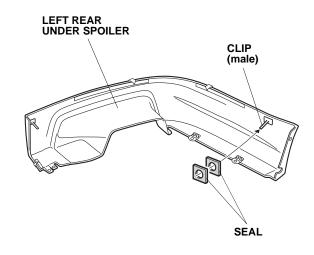
10. Using isopropyl alcohol on a shop towel, clean the surface where the left rear under spoiler will attach.
