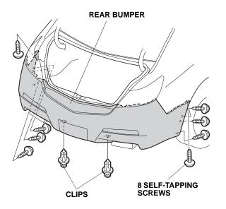
• On each side, release the twelve hooks, and gently pull the rear bumper away from the body.
