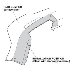
12. Install the left rear under spoiler on the rear bumper using two fender bolts and one bumper bolt, and loosely install the three washer nuts.
