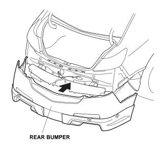
17. Remove the six adhesive backings in the order shown below. While pressing the rear under spoiler firmly against the rear bumper with the palm of your hand, carefully remove each adhesive backing.
