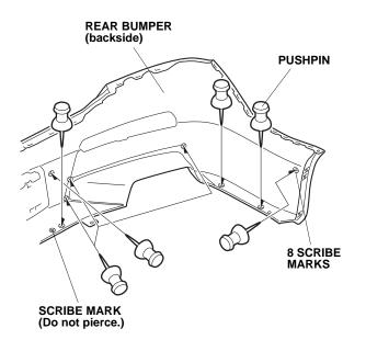
3. While wearing eye protection, drill the eight pierced marks using a 3 mm drill bit, then finish with a 10 mm bit.
