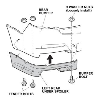
13. Loosely install the one self-tapping screw to the left rear under spoiler.
