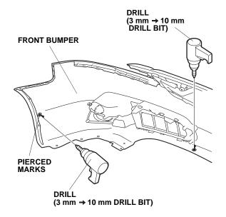
From the outside (painted side) of the bumper, drill the remaining pierced mark to 10 mm. First drill with a 3 mm drill bit, and finish with a 10 mm drill bit.
