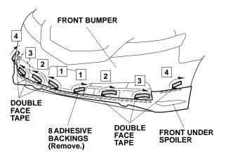
28. Using a hard rubber roller, apply pressure and roll it from one end to the other.
