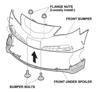
21. Install two bumper bolts on the front under spoiler, and loosely install the two flange nuts.
