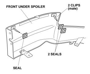
20. Install the front under spoiler on the front bumper.
