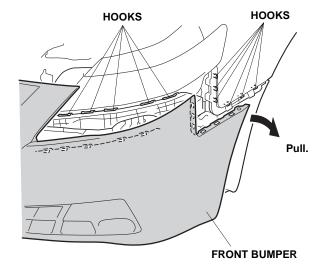
10. With the help of an assistant, remove the front bumper (two vehicle clips and unplug the five vehicle connectors). Place the front bumper on the blanket to prevent damage.
