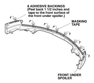
18. Using isopropyl alcohol on a shop towel, clean the bumper where the front under spoiler will attach.
