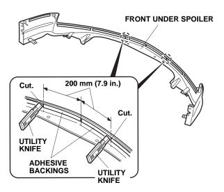
17. Peel back approximately 1-1/2 inches of adhesive backing, and tape the ends to the front surface of the front under spoiler.
