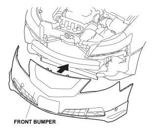
26. On each side, install the one self-tapping screw to the front under spoiler.
