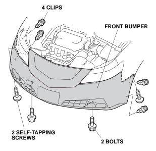
9. On each side, release the eleven hooks, and pull the front bumper out from the body.
