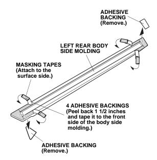
Clean the door surface where the left rear body side molding will attach using one alcohol pad. Allow the alcohol to dry.
