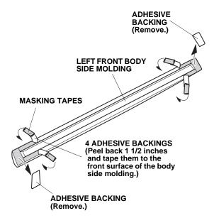
3. Clean the door surface where the left front body side molding will attach using one alcohol pad. Allow the alcohol to dry.
