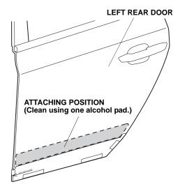
11. Install the left rear body side molding on the left rear door, aligning the edges of the left rear body side molding with the edges of the rear template as shown.
