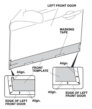
Peel back approximately 1-1/2 inches of adhesive backing from each adhesive tape, and tape the ends to the front surface of the left front body side molding. Remove the small end pieces of the adhesive backing.
