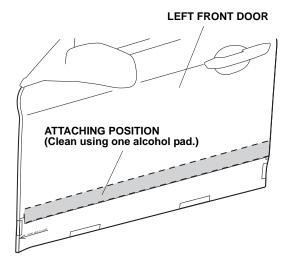
4. Install the left front body side molding on the left front door, aligning the edges of the left front body side molding with the edges of the front template as shown.
