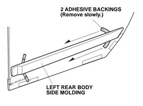
13. Using the rubber roller, apply firm pressure while rolling to set the adhesive.
