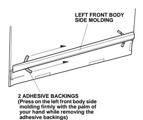
6. Using the rubber roller, apply firm pressure while rolling to set the adhesive.
