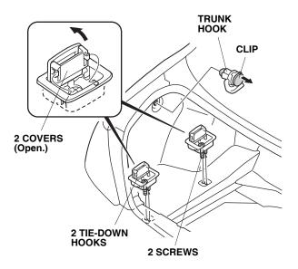
25. Pull away the weatherstrip, and remove the left trunk side trim panel (two clips).
