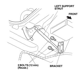
30. Have an assistant hold the trunk lid. Using a 12 mm open end wrench, remove the support strut by removing the stud ball. Open the trunk lid halfway to remove the stud ball.
