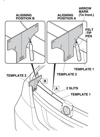
4. Turn over template 1. Align template 1 with the "A" emblem and the right edge of the trunk lid. Secure template 1 with masking tape starting from the center and working toward the right edge of the trunk lid.
