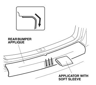
11. Use the applicator with soft sleeve to apply the rear bumper applique to the rounded rear edge on the left side as shown. Start in the middle and work outward. Repeat for the right side. 12. Remove the protective film from the top rear bumper applique. Slowly pull the protective film back. Avoid pulling it upward.
