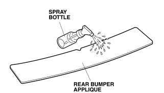
6. Wihout touching the adhesive side of the rear bumper applique, position it on the rear bumper, and align the v-notch in the rear bumper applique with the center of the trunk lid anchor. Smooth the rear bumper applique along the rear bumper and tape each end at the curved surface.
