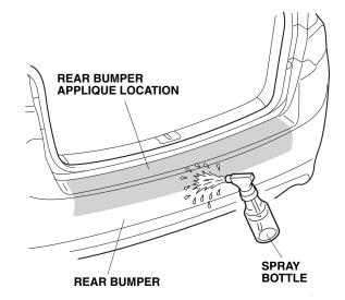
4. Remove the adhesive backing from the rear bumper applique.
