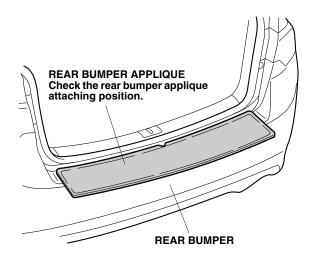
2. Using isopropyl alcohol on a lint-free shop towel, clean the rear bumper where the rear bumper applique will attach. Remove the rear bumper applique.
