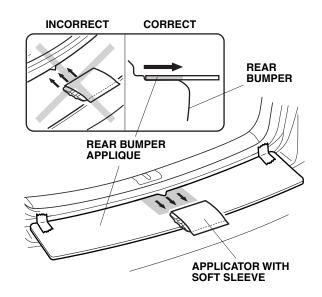
8. Starting from the center and working outward, use the applicator with soft sleeve to smooth the rear bumper applique. Repeat on the right side. Stroke in one direction only.
