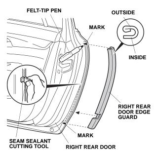
11. Position the cutting edge of the seam sealant cutting tool against the door edge, and trim the seam sealant from mark to mark between the marks at the top and bottom of the door edge.
