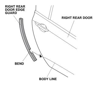
10. Using a felt-tip pen, mark the inside edge of the right rear door at the upper and lower ends of the right rear door edge guard.
