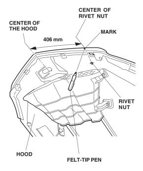
7. Using an alcohol swab, clean the area where the protective tape will attach. Attach the protective tape around the front edge of the hood starting at the location shown.
