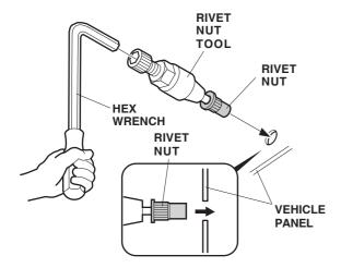
Holding the rivet nut tool with the hex wrench, turn the 19 mm wrench clockwise and install the rivet nut on the vehicle panel.
