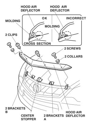
15. Open the hood, and check that there is no clearance between brackets B and the hood.
