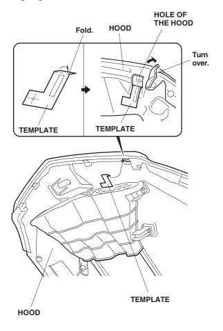
3. Using a felt-tip pen, mark the hood as shown. Remove the template.
