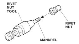
Insert the rivet nut into the hole in the vehicle panel and install the hex wrench on the rivet nut tool.
