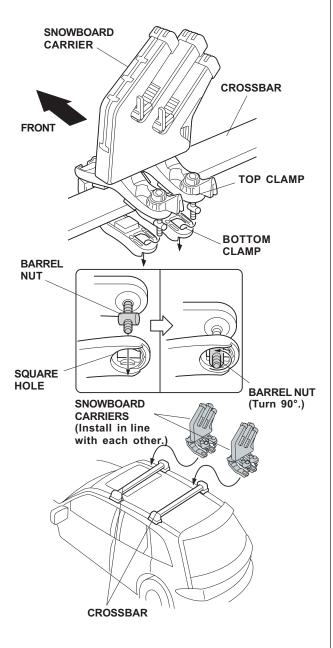
8. Turn the four knobs on the four top clamps to tighten the snowboard carrier.
