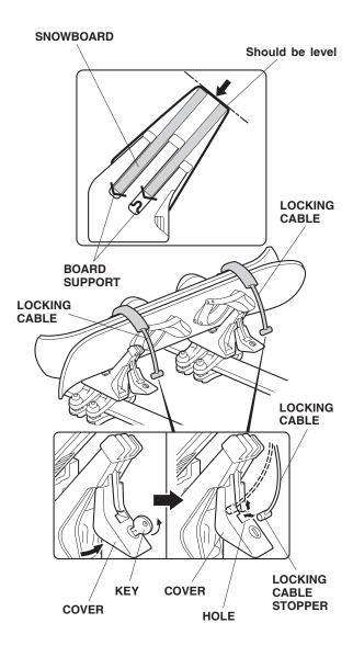
14. Check that the locking cables are installed securely, then close the covers.
