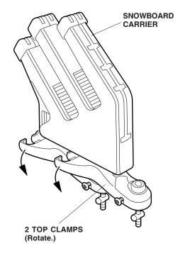
Install two board supports to the snowboard carrier.
