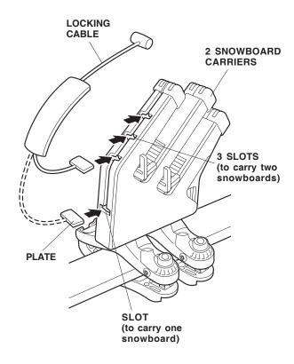
13. After loading the snowboard(s) on the carrier, adjust it (them) with the help of the board supports so that the top edges are level and the boards are as far down in the carrier as possible. To secure the snowboard(s), use the key to open the covers, then insert the locking cable stoppers into the holes of the carrier covers.
