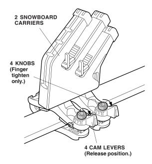
9. Return the four cam levers to the original location (turn clockwise).
