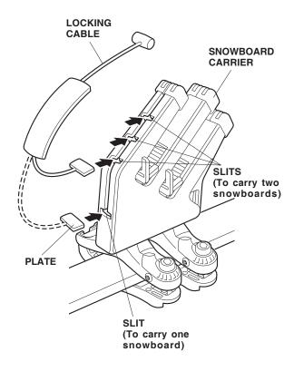
15. After loading the snowboard(s) on the carrier, adjust it (them) with the help of the board supports so that the top edges are level and the boards are as far down in the carrier as possible. To secure the snowboard(s) use the key to open the covers, and insert the locking cable stoppers into the holes in the carrier covers.
