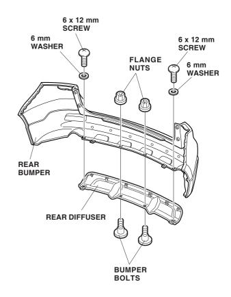
11. Secure the rear diffuser to the rear bumper using six 5 x 12 mm self-tapping screws and six 5 mm washers.
