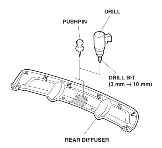
2. While wearing eye protection, drill a 10 mm hole at each pierced mark. First drill with a 3 mm drill bit, and finish with a 10 mm drill bit.
