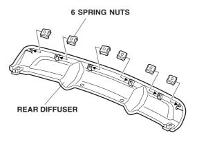
10. Install the rear diffuser on the rear bumper using two 6 x 12 mm screws, two 6 mm washers, two bumper bolts, and two flange nuts.
