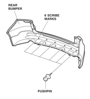
7. While wearing eye protection, drill a 3 mm hole through each marked location on the bumper. Enlarge the inner holes to 11 mm using an 11 mm drill bit. Enlarge the outer holes to 8 mm using an 8 mm drill bit. Remove any burrs from the edges of the holes with a file.
