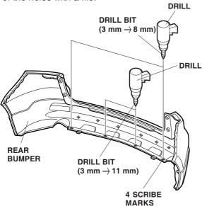
8. While wearing eye protection, drill a 3 mm hole through each marked location from the inside of the bumper, and finish with a 6 mm drill bit. Remove any burrs from the edges of the holes with a file.
