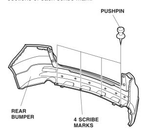
6. Inside the bumper, locate the six scribe marks in the area shown. Using a pushpin, pierce the cross sections of each scribe mark.
