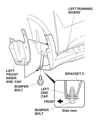
While pushing up on the running board, secure the left front inner end cap with the three long selftapping screws.
