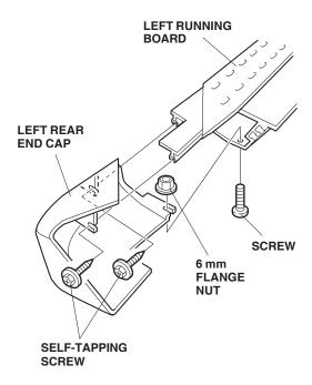
5. Align the bolts on the left running board to the holes in the Brackets A and B you just installed on the side sill trim, and install it by loosely tightening six 8 mm flange nuts.
