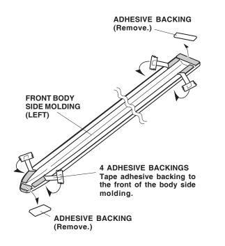
Using one alcohol pad, clean the area where the 4. side molding will attach.
