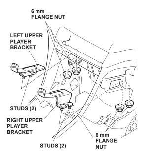
11. Remove the two nuts from the premium sound system amp.
