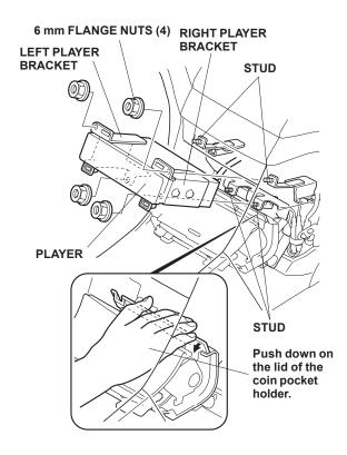
20. Insert two player panel hooks into the square holes of the right and left player brackets, then insert two player panel clips into the latches.
