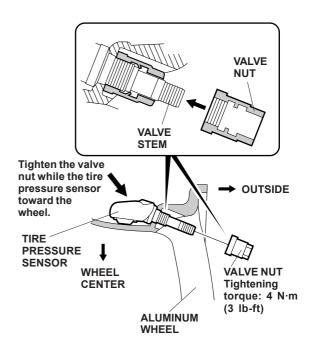
4. Tighten the valve nut to the specified torque while holding the tire pressure sensor toward the wheel. You may hear a snap or pop as you tighten the nut. This is normal.
