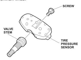
3. Install the tire pressure sensor to the aluminum wheel and loosely install the valve nut. Make sure the pressure sensor is resting on the wheel.
