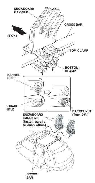
8. Turn the knobs on the top clamp to tighten the front carrier.
