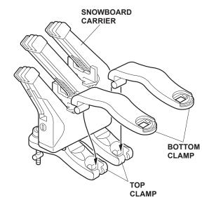
Repeat steps 1 thru 5 to assemble the other carrier. 7. Attach one carrier to the front cross bar in the direction shown. Insert the barrel nuts on the top clamp into the square holes in the bottom clamp, and turn the nuts 90° to lock them into position. Install the other carrier to the rear cross bar using the same procedure. Make sure the rear cross bar is parallel to the front cross bar.
