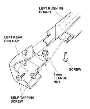
5. Align the bolts on the left running board to the holes in the Brackets A and B you just installed on the side sill trim, and install it by loosely tightening the six flange nuts.
