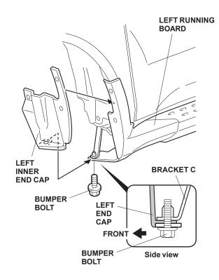
7. While pushing up on the running board secure the left inner end cap with the three long self-tapping screws.
