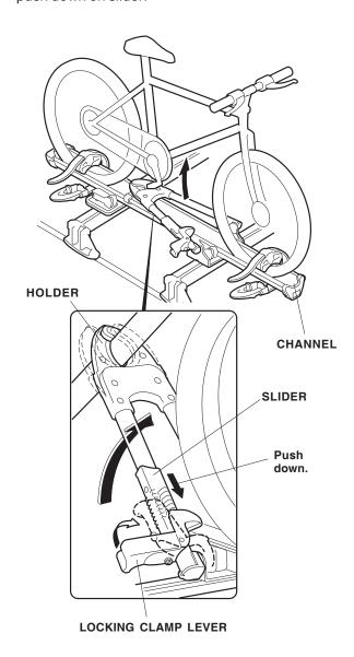
3. Push up the locking clamp lever to secure the bicycle's frame.
