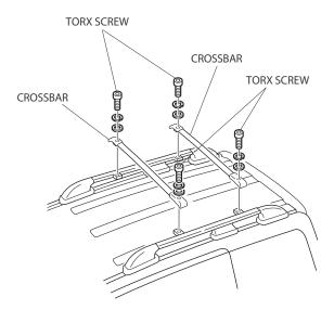
10. Using a T-25 Torx driver, remove the Torx screws from one end of the roof rack crossbars (front and rear). Remover the end cap. Remove the roof rack end caps from the same side of the vehicle.
