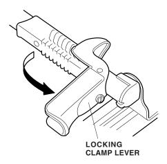
14. Turn and adjust the mounting lever to lock the bicycle attachment to the roof rack. Check for firm pressure while you push down on the mounting lever to lock it into place.
