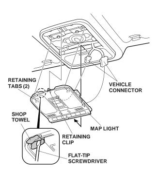
4. Remove the roof console (four screws).
