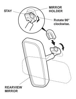
6. Replace the clip. Slide the day/night mirror stay onto the mirror holder, then turn the mirror counterclockwise as shown.
