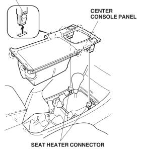
4. Open the pocket lid. Pull the pocket out toward you to release the four clips, unplug the illumination bulb, unclip the illumination bulb harness from the pocket, and remove the pocket. Take care not to damage the illumination bulb.
