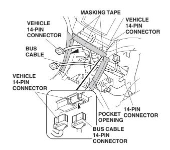
8. Wrap one wire tie with clip around the bus cable, and push the wire tie with clip into the hole in the vehicle frame.
