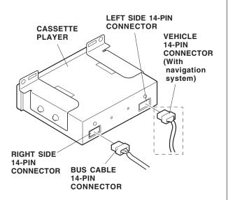
19. While pushing down on the coin pocket or ashtray holder, install the player into the dash opening and onto the studs of the upper player brackets. Install one 6 mm flange nut on the end of each stud. Tighten the flange nuts securely.
