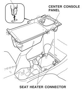
4. Open the pocket lid. Pull the pocket out toward you to release the four clips, unplug the illumination bulb, unclip the illumination bulb harness from the pocket, and remove the pocket. Take care not to damage the illumination bulb.
