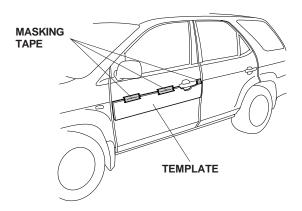
Repeat steps 2 and 4 to install the rear template to the rear door.
