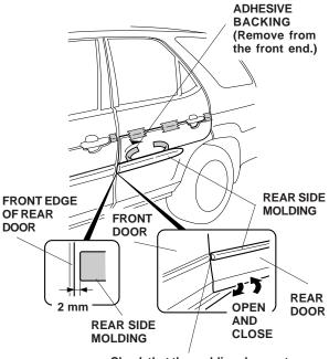
Check that the molding does not interfere with the front door when the rear door is opened and closed.
