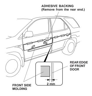
While holding light pressure against the molding, slowly and carefully remove the adhesive backing starting at the rear and working toward the front. Hold the molding firmly against the door panel with the palm of your hand for 30 seconds.
