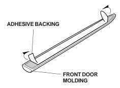
Position the molding on the door panel and align the upper edge of the molding with the lower edge of the template. Adjust the location so that there is a 2 mm gap between the rear edge of the molding and the front door.
