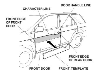
While holding the template in position, apply masking tape in the areas shown.
