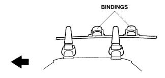
3. Close the top frame. While holding the top frame firmly against the ski/snowboard, lock the top frame by turning the key couterclockwise.
