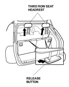
3. Store the headrests in the storage compartment under the cargo floor. Insert the shafts of the headrests into the holes in the sides of the storage compartment.
